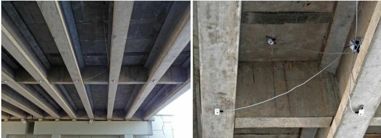
Figure 1 - General view of the installation (left) and weight sensors (WM), shear stress (WC) and Free-of-Axle Detectors (FAD) sensors (right).
