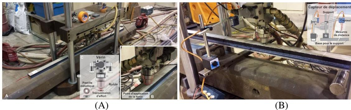
**Figure 1 – In (A) details of the punching test, in (B) the details of the three-point bending test**
