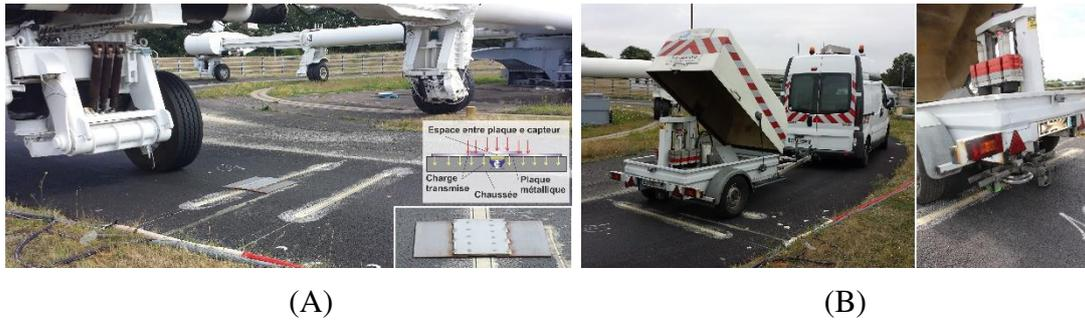
**Figure 4 – The image (A) shows the metal plate covering one sensor, the plate details and alignment with sensor, in the image (B) show the FWD trailer positions relatively to the sensor**
