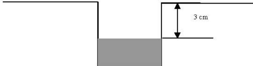
Place the sensor in the middle of the cutting and use some weight to maintain it in place without bending it. Continue to work on the resin until there's no more resin overflowing on the tape. Ensure there's no air between the resin and the sensor, remove all the air bubbles.
