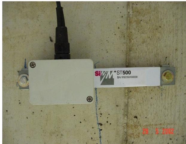
Figura 11 – Sensor SiWIM (strain gauge) instalado
